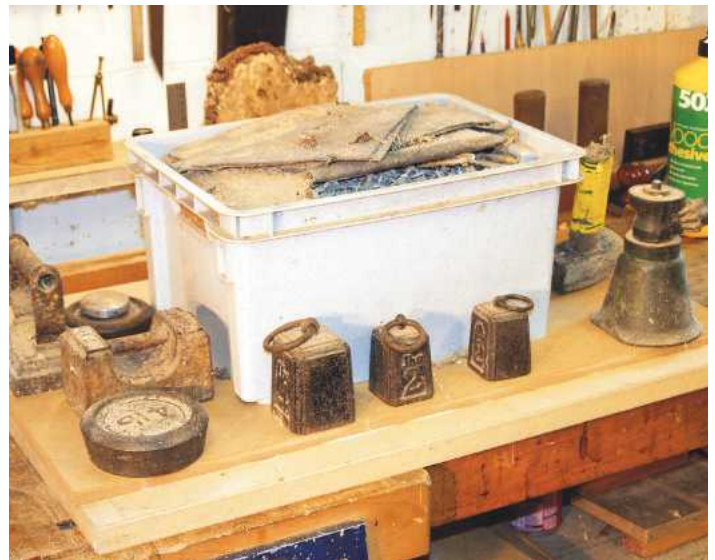
▲ Pic.9 Place the top board in position and weigh it down with every heavy object you have; make sure it doesn't slide out of position
